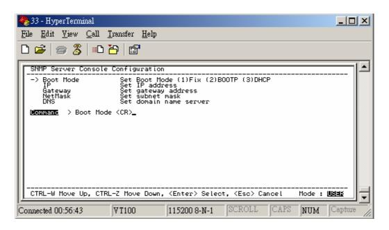
15. Enter in the IP Address, the Gateway Address, the Subnet Mask and the DNS (all required). Hit the "Escape" key to return to the main menu.
